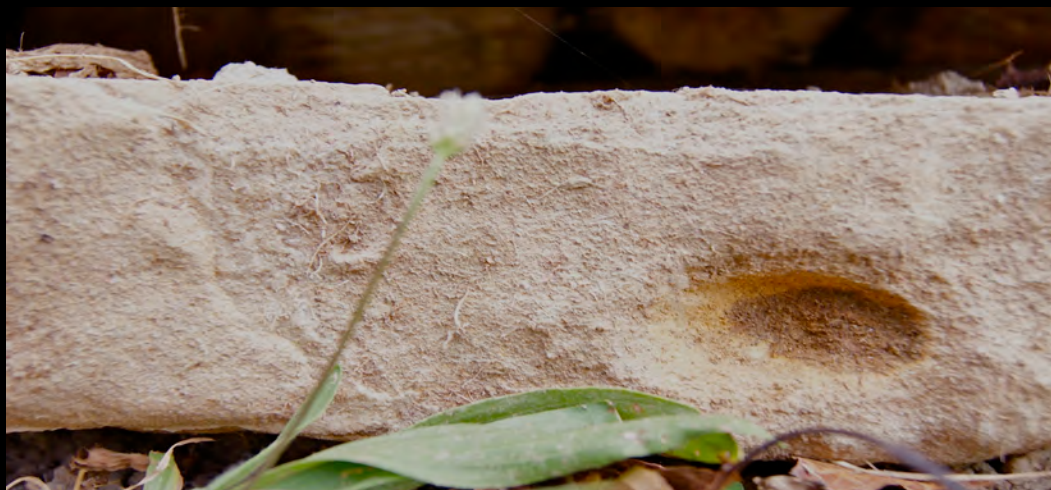
Kopaci Block- Exposed 'vein' surface oxidation
