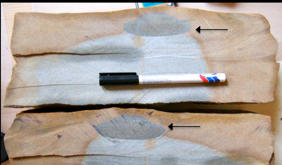
Sectional cut displaying Vein in upper centre of Block
