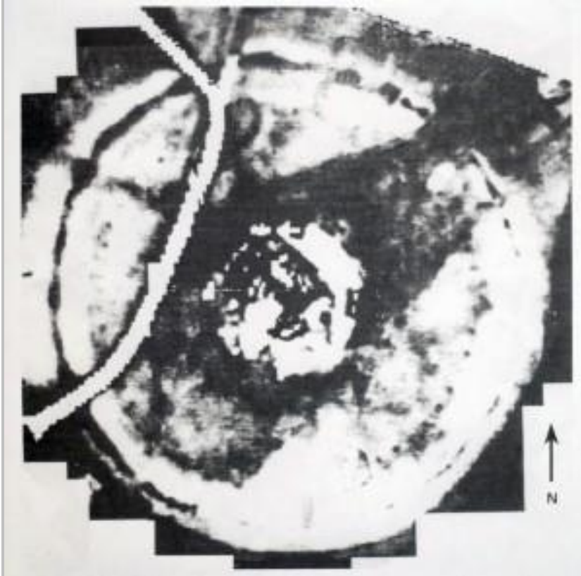
Fig. 21. Electrical resistivity map of the ground at Stonehenge. Darker shading suggests earth that has had more natural electrical run through it. Poor conductivity of the ring-shaped ditch forces the current to concentrate in the gap of the causeway entrance at the northeast. Inside, it fans out and hugs the stone circles (bright ring at center). The white, curving line to the left is the modern, paved visitors' path. (After R.M.J. Cleal, K.E. Walker, and R. Montague. Stonehenge and Its Landscape , p. 499. © by English Heritage, London, 1995)
